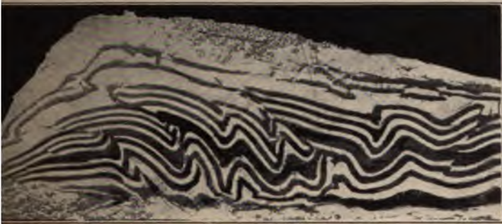
experimental production of a series of parallel thrusts within closely folded strata (after Willis).
